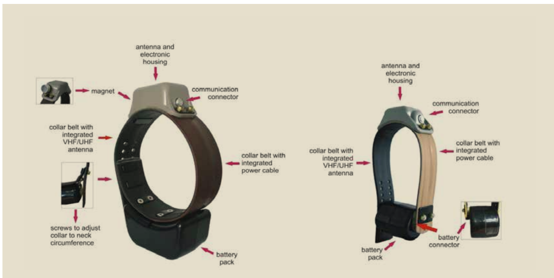
Figure 25: Radio - collars and Different Components
